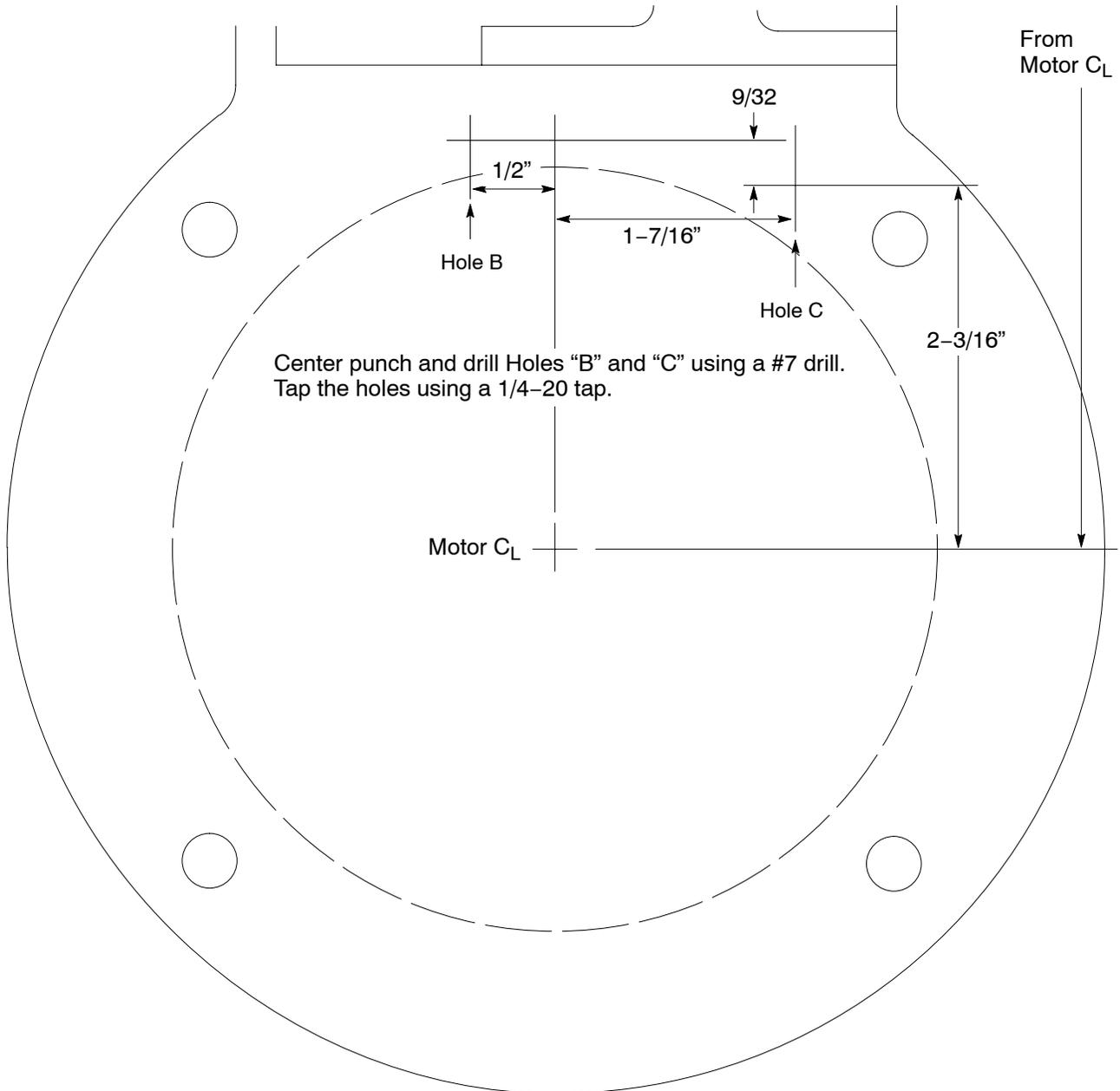
Figure 4 Guard Kit Assembly Diagram
