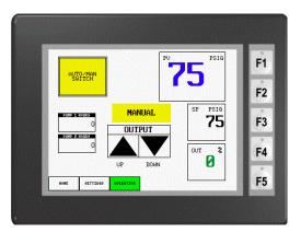
The Operating Screen is used to set the controller for Auto/Manual Operation and System Setpoints. Pressing the Auto/Manual switch provides a bump less transfer between Auto & Manual system operation.
