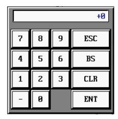
Enter the desired set points and press **ENT** to save the setting. The new setting will be displayed on the button. To exit the data entry box press **ESC** button.
