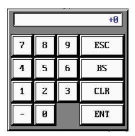
Enter the desired set point and press **ENT** to save the setting. The new setting will be displayed on the button.
