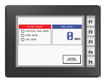
The controller Main Screen Provides the level in the tank level and System Alarms.
