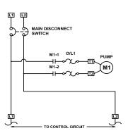
Standard Motor Controls Incoming Power Service of 200/240vac - 1 phase. Simplex and Duplex setup (Figure 2). Adder Options Available.
