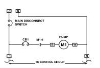
Standard Motor Controls Incoming Power Service of 115/120vac - 1 phase. Simplex and Duplex setup (Figure 1). Adder Options Available.
