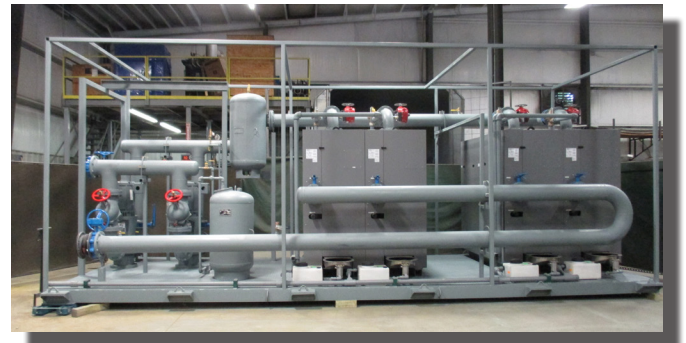
FIGURE 1. Four (4) boiler envirosep PBS modular skid
