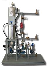
designed to address the requirements of commercial potable water heating systems. Designed to utilize steam as the heat source, the steam is supplied to the heater at a predetermined 2 to 60 psig (depending on required output). The *envirosep IWH* is constructed of stainless steel, copper, and bronze components suitable for domestic water use. Capable of handling a wide range of water flow rates (5 to 300 gpm) and
