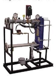
of hot water, resulting in less square footage required for mechanical equipment. An internal circulation pump is provided to obtain an even temperature profile throughout the heater. The envirosep IWH-PF, instantaneous water heater with plate & frame design, may be manufactured to include a system recirculation pump, which is recommended for maintaining hot water loop temperature. Electrical controls
