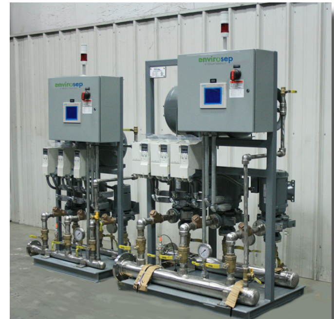
FIGURE 1. Space saving custom duplex and triplex envirosep DBS, domestic water booster systems, with close coupled end-suction pumps and hydro-pneumatic tank.
