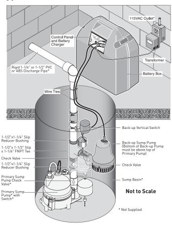
\* Deep cycle marine-type battery (Group 24) recommended – not included with FG-100 system
