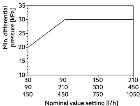
For the variants DN 10 LF, DN 15 LF (both 30 to 210 l/h), DN 10 (90 to 450 l/h) and DN 15 (150 to 1050 l/h) the measured differential pressure is not identical to the actual differential pressure P1-P3.
