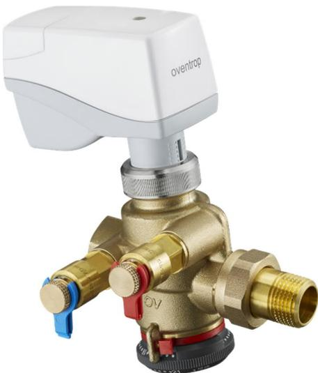
Pressure independent control valve for dynamic hydronic balancing of heat exchangers, for example fan coils or cooling ceilings and distribution pipes in heating and cooling systems with closed circuits. The valve combination consists of an automatically operating flow controller and a control valve and can be equipped with an actuator or a manual regulating head. Installation in the supply or the return pipe.
