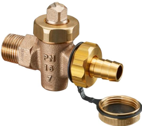
Based on DIN 3848. For liquids, steam and treated heating water, e.g. district heating. Can be used up to 180 °C for short periods. The fill and drain cock is opened/closed with a 90° rotary movement. The switching position is marked on the top of the square.
