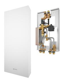
For the supply of individual dwellings with heating water and hot potable water. The required heat is provided by a central heat supply. Hot potable water is prepared decentrally via a plate heat exchanger according to the continuous flow principle. When selecting the dwelling station, it is necessary to consider the water quality of the area of use.
