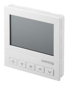
The room thermostat is used for individual temperature control of two-pipe systems. The room temperature is controlled via a valve which is controlled by the room thermostat via a thermal actuator. When the room temperature reaches the setpoint temperature, the valve is closed. In addition, the room thermostat enables the electrical control of fan coil units for demand-oriented heating or cooling.
