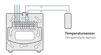
The ClimaCon F temperature sensor is used as an external temperature sensor to detect the temperature in the room or the surface temperature as limiter.
