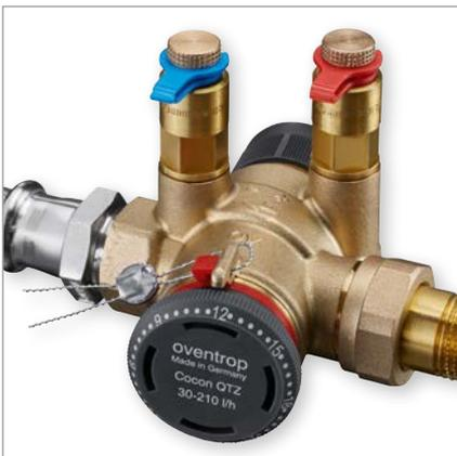
The setting is protected against unauthorised tampering with the help of the handwheel which engages automatically. The setting can be additionally secured by inserting the red locking ring which can be lead sealed. Even with the actuator in place, the settings of the “Cocon QTZ” can be read off and adjusted.
