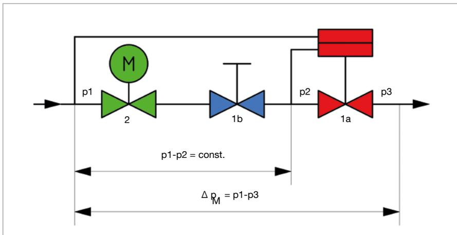
The **integrated diaphragm unit** (pos. 1a) keeps the differential pressure “p1”-“p2” at a constant level via the regulating unit (pos. 2) which is activated through the actuator and via the nominal value unit (pos. 1b) which can be set to a maximum flow value. Even where high differential pressure variations “p1”-“p3” occur, e.g. if sections of the system are activated or inactivated, the differential pressure “p1”-“p2” is kept at a constant level.
