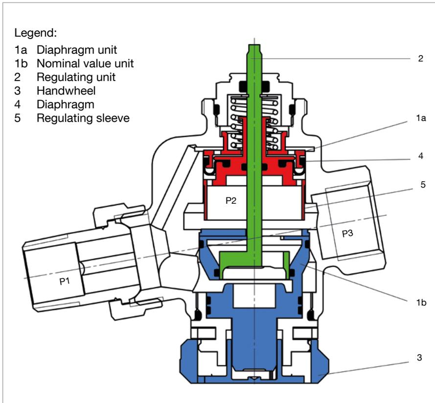
The required **flow rate** is set with the help of the handwheel (pos. 3). The illustrated section shows three pressure ranges: “p1” is the inlet and “p3” the outlet pressure of the valve. “p2” is the pressure actuating the diaphragm unit (pos. 1a) which keeps the differential pressure “p1”-“p2” at a constant level.
