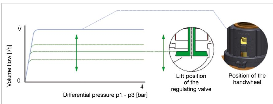
The maximum volume flow ( $\dot{V}$ ) within the control range (0.2 - 4 bar) is set with the help of the handwheel. During low demand periods, the volume flow is regulated to the required value by the lift position of the regulating valve.
