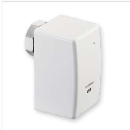
Electromotive actuator with connection thread M 30 x 1.5, system EIB, with integrated bus coupling. The electromotive actuator EIB is suitable for the direct connection to the European installation bus control system. The power absorption is extremely low, so that a separate power supply is not needed.
