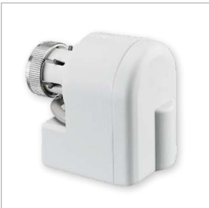
Electromotive actuator with connection thread M 30 x 1.5. For room temperature control in conjunction with two point controllers. For use in radiant and chilled ceiling systems as well as induction air systems.
