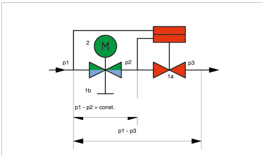
The **integrated diaphragm** unit (pos. 1a) keeps the differential pressure “p1”-“p2” at a constant level via the regulating unit (pos. 2) which is activated through the actuator and via the nominal value unit (pos. 1b) which can be set to a maximum flow value. Even where high differential pressure variations “p1” - “p3” occur, e.g. if sections of the system are activated or inactivated, the differential pressure “p1” - “p2” is kept at a constant level.
