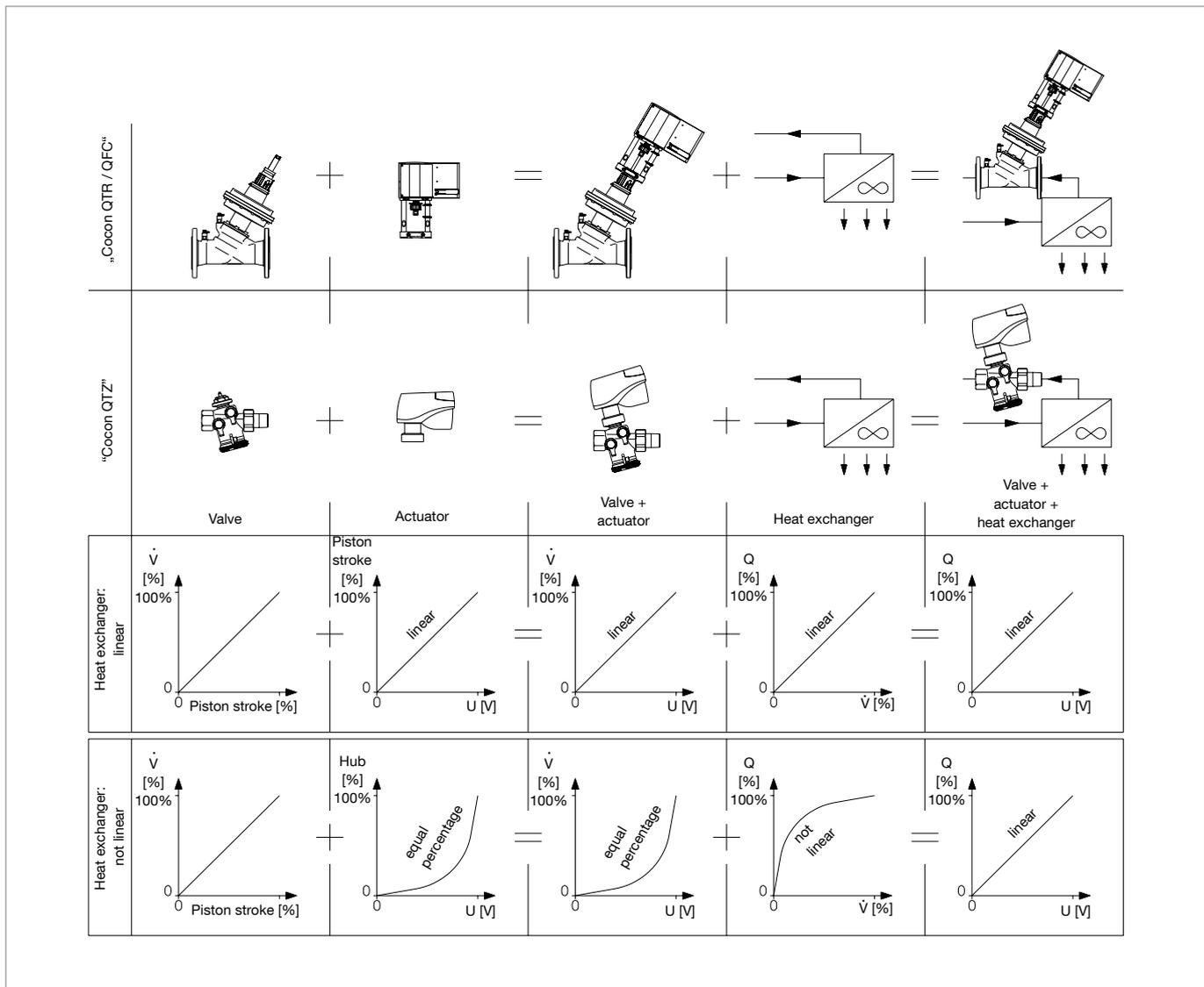
Optimisation of the interaction of valve, actuator and heat exchanger with modulating 0-10 V actuators. The illustration shows idealised characteristic lines explaining the control principle.
