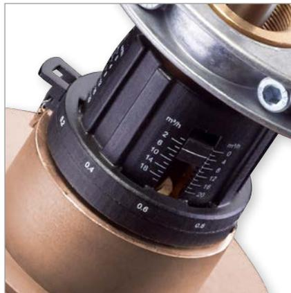
The nominal values are imprinted on three peripheral scales ensuring an excellent optical display of the values in any installation position. The nominal values can be set in m<sup>3</sup>/h. The locking clip can be lead sealed to secure the setting from unauthorized access.
