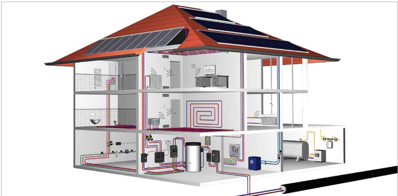
**The variety and different models of Oventrop valves and controls allow the stockist, plumber and specifying engineer to fulfil all technical requirements concerning radiators, accessories and the complete heating system. Due to their presetting, they permit a hydronic adjustment of the flow rate and thus guarantee an economical heat output of the individual radiators.**
