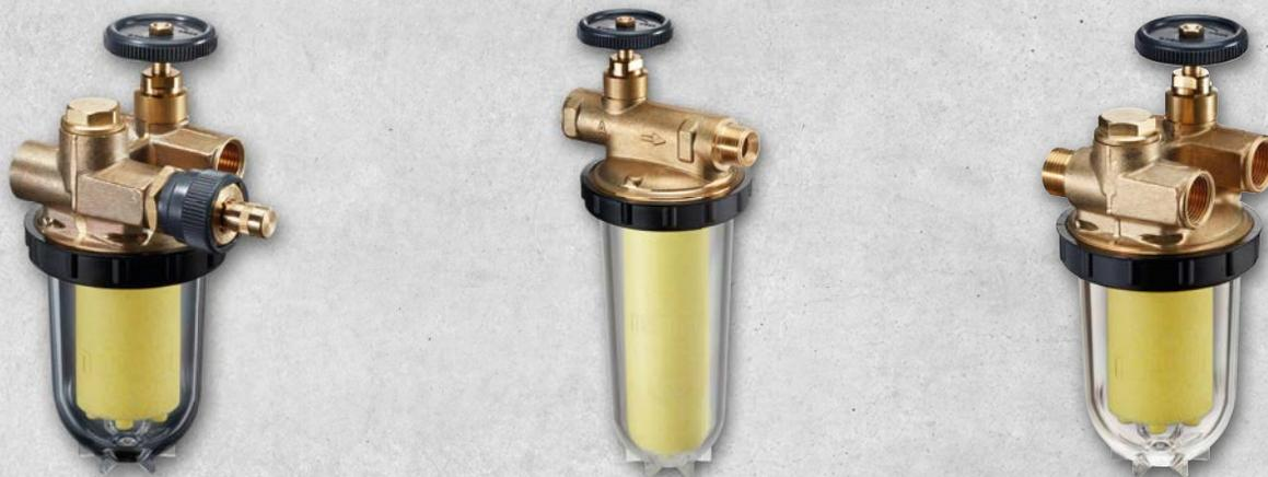
Heating oil **filters Oilpur** are used in oil firing systems that are operated as one pipe system with or without return flow feed or as two pipe systems. Filters with *plastic filter cups* are generally only approved *for suction operation*. *Metal filter cups and the filter cartridge* are also approved for *pressurised systems* and are available optionally or as accessories.
