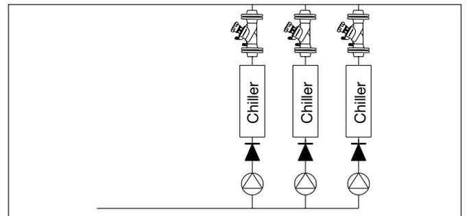
Example: Cooling system with flanged connections.
