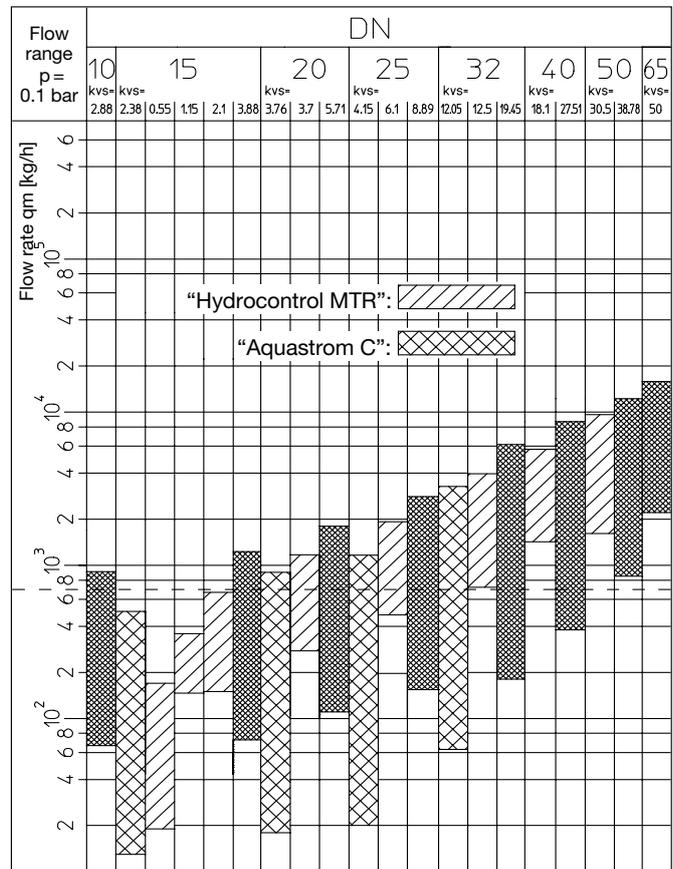
Flow ranges between lowest and highest presetting with  $p = 0.1$  bar via the double regulating and commissioning valve.
