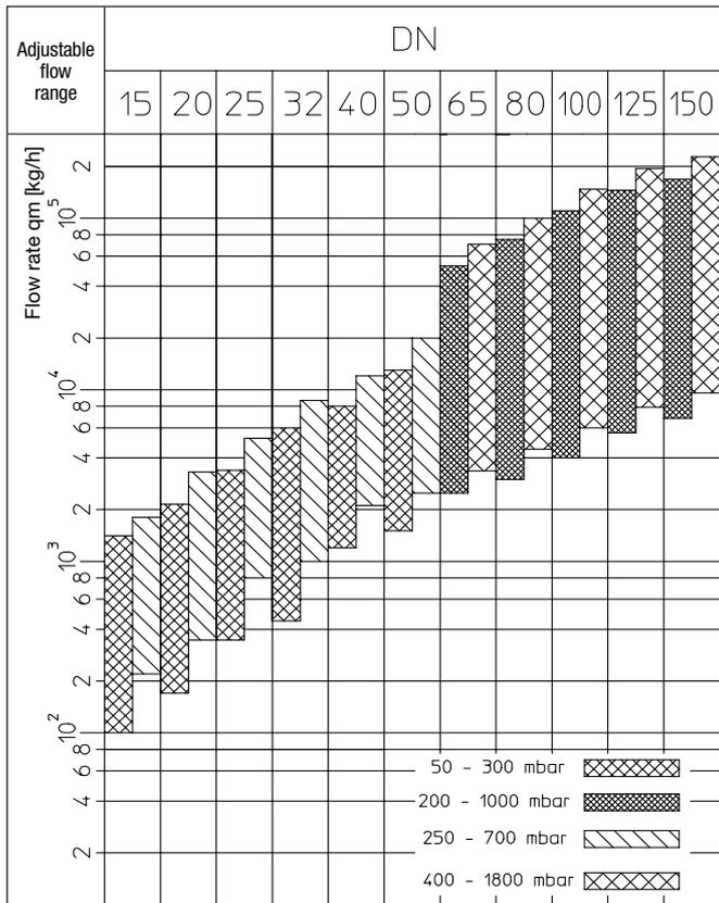
Flow ranges of the differential pressure regulator “Hydromat DTR” for adjustable differential pressures in the circuits 50–300 mbar or 250–700 mbar. For the “Hydromat DFC” differential pressures of 200–1000 mbar or 400–1800 mbar are possible. The additional flow limitation is carried out at the double regulating and commissioning valve “Hydrocontrol VTR/VFR”.
