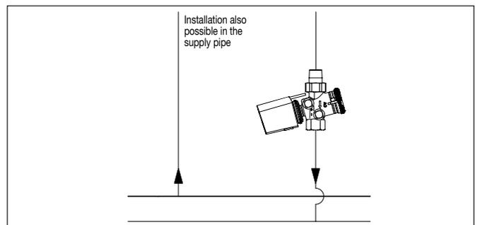
Example: Flow regulation at the pressure independent control valve “Cocon QTZ”.
