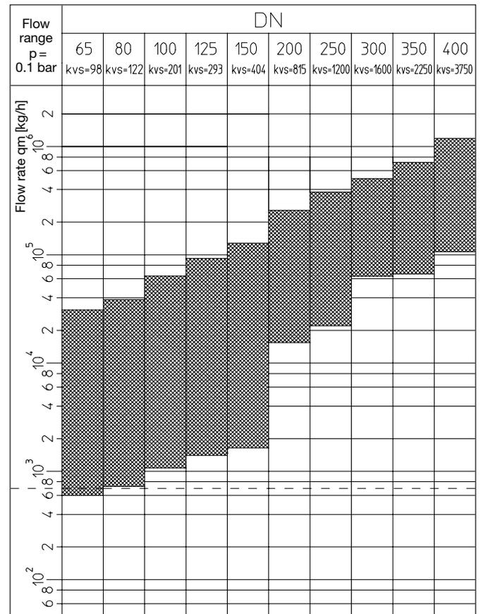
Flow ranges between lowest and highest value of presetting with  $p=0.1$  bar via the double regulating and commissioning valve. The below examples only show the valves which are really required for hydronic balancing.
