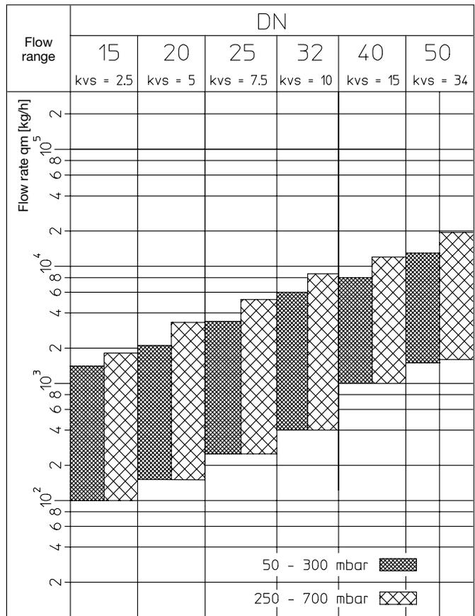
Flow ranges of the differential pressure regulator “Hyocon DTZ” for adjustable differential pressures in the circuits 50–300 mbar or 250–600 mbar
