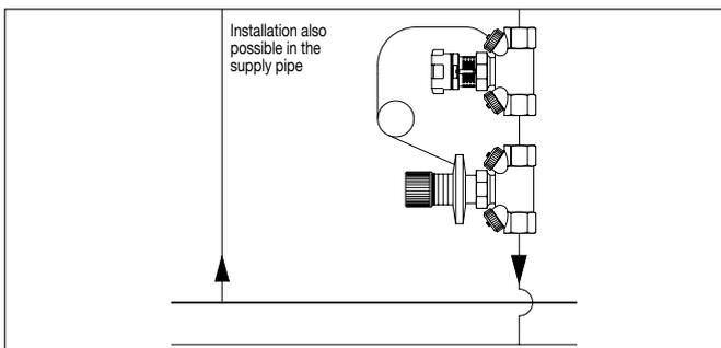
Example: Flow regulation with the help of the combination differential pressure regulator “Hycocon DTZ” and double regulating and commissioning valve “Hycocon VTZ”.
