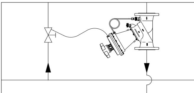
Example: Differential pressure regulation in installations with flanged connections.
