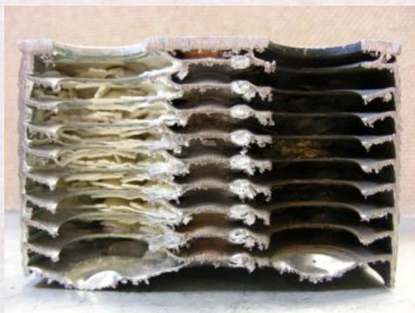
Figure 10. Fouling and clogging of a heat exchanger.
