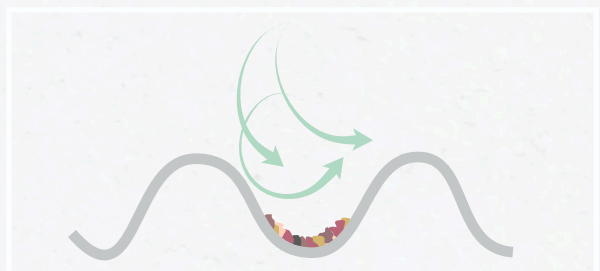
Figure 8: The effect of increased shear stress on fouling.
