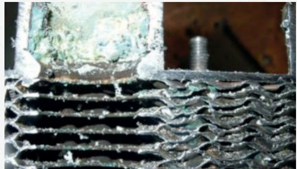
Figure 6: Limescaling in a heat exchanger
