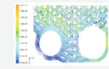
Simulation is one of the most important stages in the development of new and existing BPHEs. The ability to evaluate different plate patterns by simulating flow rate and directions offers great opportunities for improved functionality.
