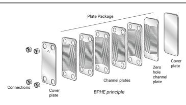
The fluids can pass through the heat exchanger in different ways. For parallel flow BPHEs, there are two different flow configurations: co-current or counter-current.
