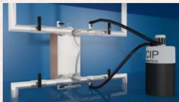
Figure 9: CIP, Cleaning in Place.
