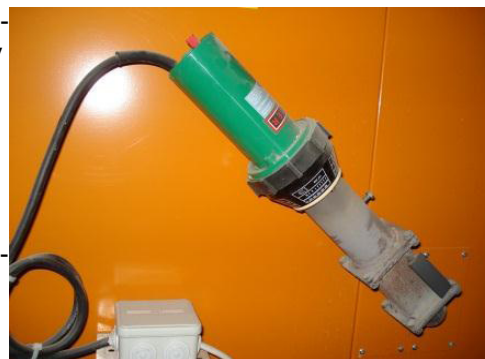
Fig. 7 Automatic ignition unit
