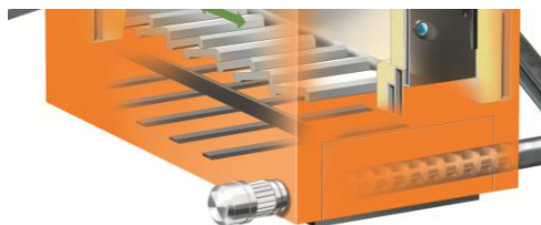
Fig. 9 Under-grate de-ashing system
