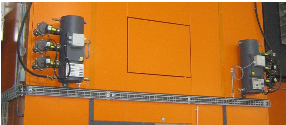
Fig. 8 Combustion system with automatic radiation-vault cleaning system
