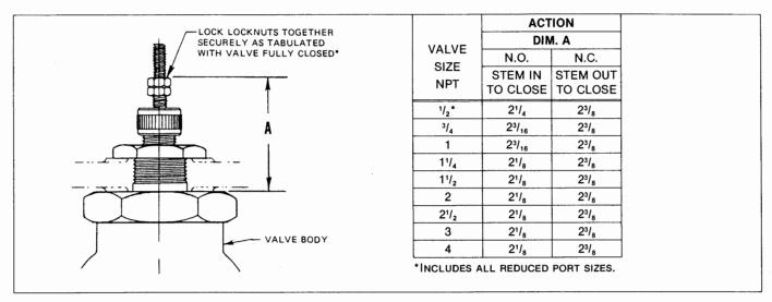
\*For 915 3-Way — Dim. A is 2 3/8 through 2" size with stem out (Top Seat Closed). Dim. A is 3" on all flanged 915 3-way. For 910EP N.O. (Stem in to close) — Dim. A is 1 7/8.
