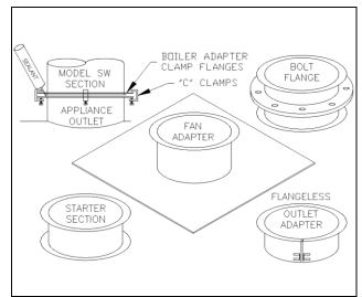
**FLANGELESS OUTLET ADAPTER - PART FOA** is a split liner piece with draw-up tabs. This adapter is intended to be slipped over a smooth collar, then drawn tight with the included fasteners.
