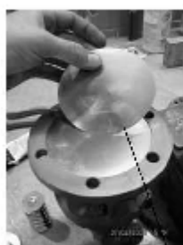
Remove & inspect diaphragms.
