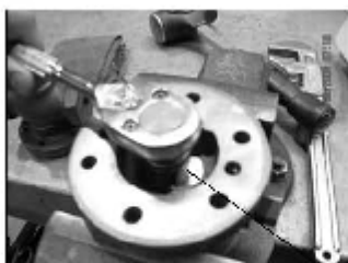
Remove and inspect pilot seal & pilot strainer.
