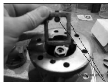
Remove pilot yoke & disc from pilot body.
