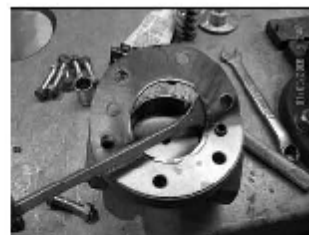
Remove any residual gasket material.
