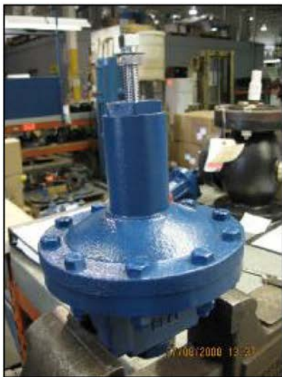
Remove valve from line.
