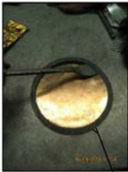
Remove gasket. (Metal diaphragms only)
