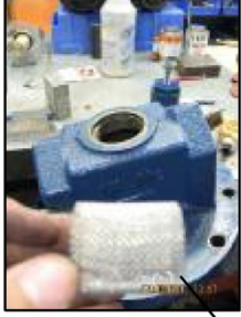
Remove, inspect and clean strainer.
