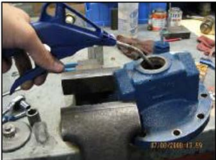
Blow debris from body and reassemble.
