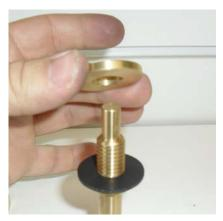
Remove disc washer and disc. Replace if necessary once stem is back in body.
