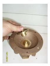
Remove diaphragm holder stem and washer.
