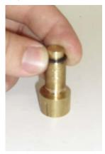
To replace O-ring, apply valve grease to threads to protect O-ring.
