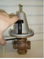
Remove all compression from main spring by turning adjustment screw counter-clockwise.
