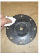
Clean and inspect diaphragm for damage. Replace if damaged.
