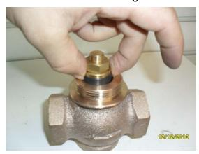
Lightly grease packing cup and carefully insert from top of valve body.
