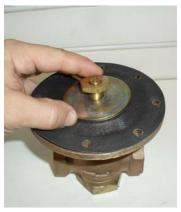
Remove diaphragm nut and washer.
