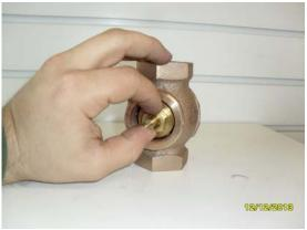
Place disc, washer, and lock nut on stem once in the body and tighten it the same way it was loosened earlier.
