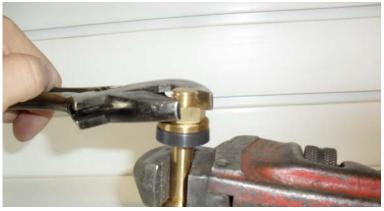
To remove the packing cup, loosen and remove packing nut as you did with the lock nut if it was not loosened during initial disassembly.
