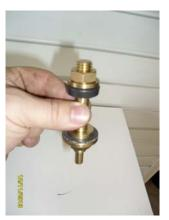
Inspect disc and packing for damage. Replace if necessary. (see next page for details)
