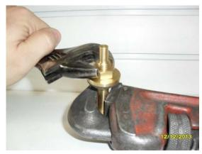
To remove disc, hold stem body with pipe wrench and loosen lock nut with appropriate wrench if the lock nut did not loosen first upon initial disassembly.
