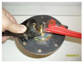
Loosen diaphragm nut by holding the unthreaded tip of the holder stem with a pipe wrench and turning the diaphragm nut counter clockwise with an appropriately sized adjustable or crescent wrench.
