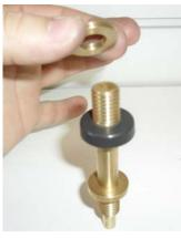
Remove packing nut, washer, and cup. Replace if necessary.
